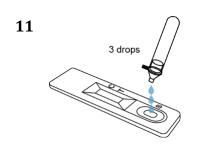
Invert the buffer tube and add 3 drops of test sample into the sample well (S) by gently squeezing the extraction tube. **Do not add to the rectangular results window.**
